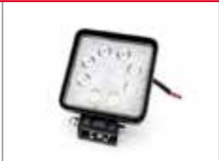
Reversing/working floodlight Version 70 W H3, 24 Volt, cable length 2500 mm 2-pin plug ASS2 Item no. 6503519
