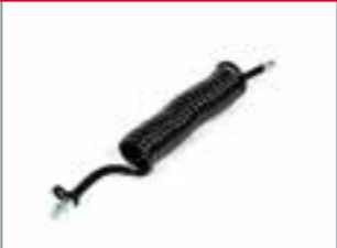
Air coil, black Anti-kink protection, black, coil: black, thread: M16 x 1.5, pipe di- ameter: 12 x 2 mm, material: TPO
