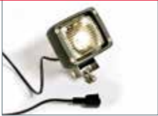
Reversing/working floodlight Version 70 W H3, 24 Volt, cable length 2500 mm 2-pin plug ASS2 Item no. 6503519
