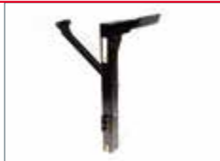
Support leg with strut Pull-out, pick-up heights 1020/1120/1220/1320 mm, Form A2 DIN EN 283/284, 18 tonnes, non-detachable bolt, shield cover Item no. 367530
