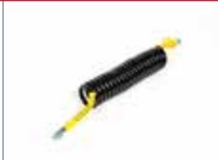
Air coil yellow Anti-kink protection: yellow, coil: black, thread: M16 x 1.5, pipe di- ameter: 12 x 2 mm, material: TPO
