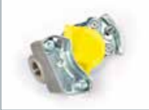
Coupling head, yellow For tractor units / with valve M16 x 1.5, OEM see 952 200 0080
