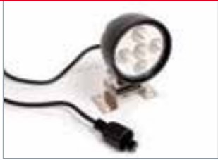
Working floodlight, round, LED LED version, 24 Volt, 500 lm, cable length 2500 mm, 2-pin plug ASS2, IP69K, approved according to ECE48/ADR Item no. 6503692
