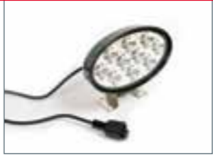
Reversing light LED version, 12/24 Volt, 800 lm, cable length 2500 mm, 2-pin plug ASS2, IP69K, approved according to ECE48/ADR Item no. 6503714
