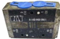
BA0018 3/2 Pilot Control Valve M14 x 1.5 Ports M10 x 1.0 Control Port Wabco OE Ref: 5710400000
