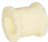
TP2465 Front/Rear Stabiliser Bush Iveco Eurocargo OE 4848464
