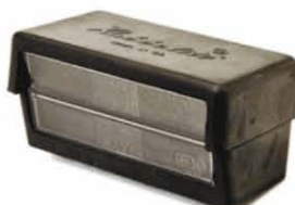
LR100/04/01 Number Plate Lamp Twin Bulb 2 x 5W LR2190 Twin Bulb Holder LR3707 Lens: 105mm x 50mm Lamp Size: 114mm x 67mm
