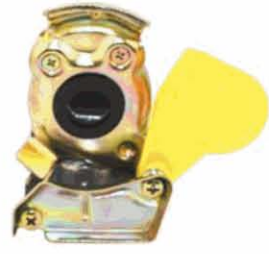
BC0597 Palm Coupling Yellow M22 c/w Self Seal Valve
