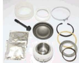
TP4040 V-Stay Repair Kit (Centre) - DAF/MAN/Volvo OE 0696320, 696320
