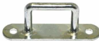
MD0555 Square Staple - Zinc Plated Steel 20mm High, 51mm Hole Centres
