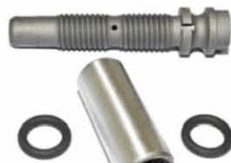
TP1035 Shackle Pin Kit - Scania 4,5,6 Series, OE 355145
