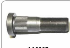
AA0007 O/L 90mm RH M22x1.5mm ISO Single To replace OE 21220132
