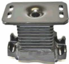
TP4010 Suspension Block DAF CF/XF OE 16995664, 1779767
